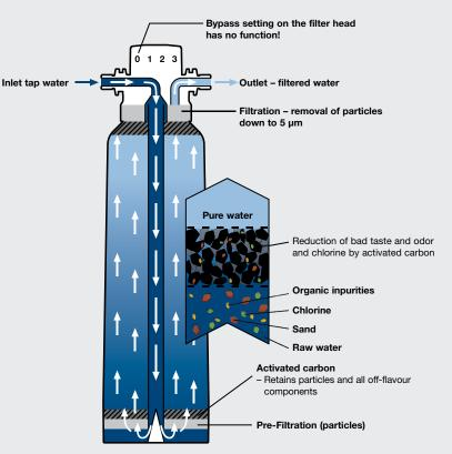
Cross-Section of a besttaste filter cartridge
